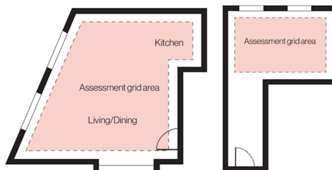
Figure 4 Assessment area examples for various room shapes
