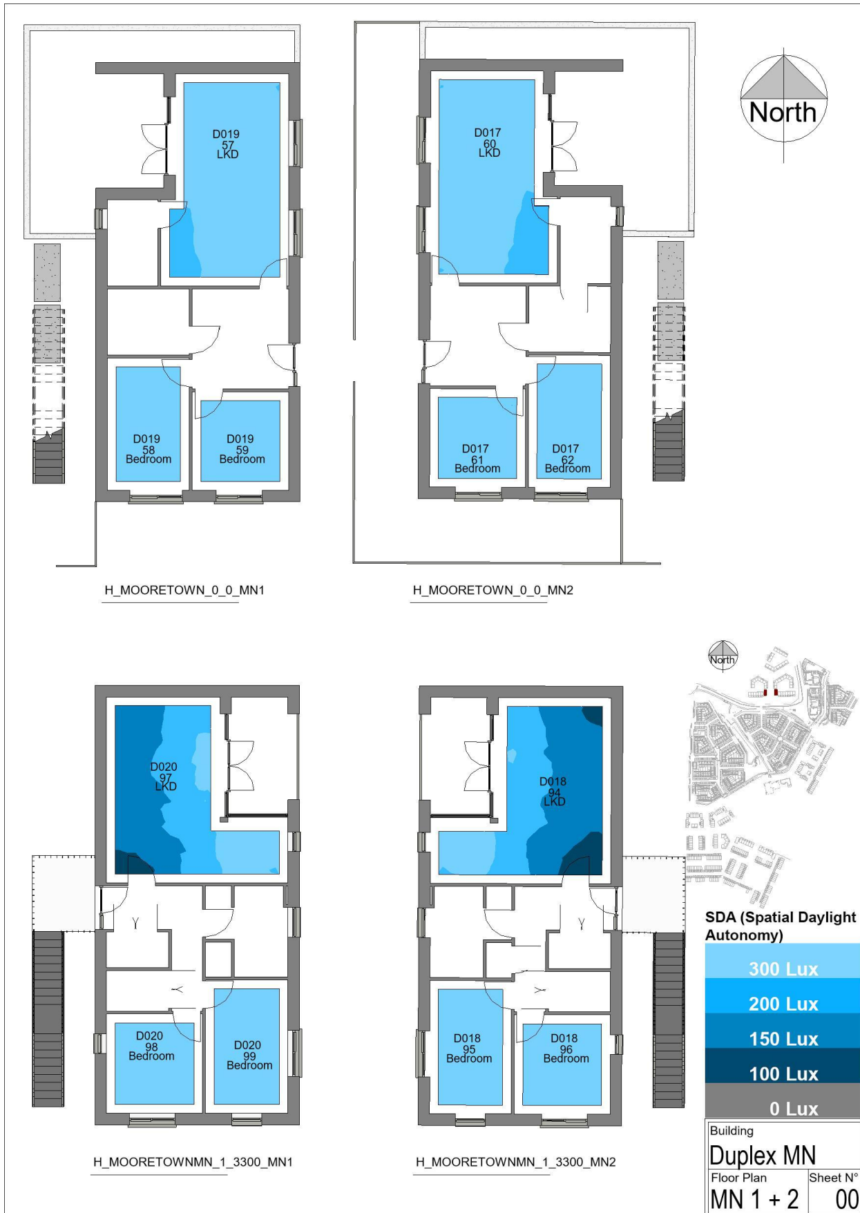
Figure 14 – Duplex Units Plans with Daylight Heatmaps
