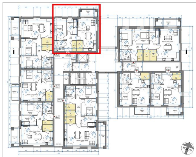
Figure 5 Apt Block Typical Floor
